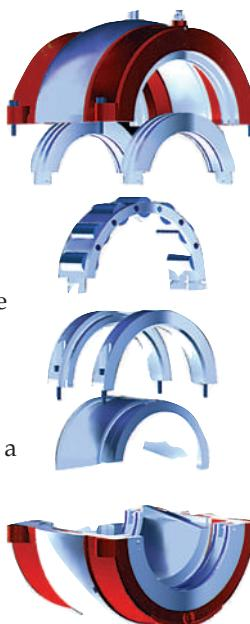
The outside diameter of the cartridge is spherically machined to accommodate initial shaft misalignment. This allows the Bearing and Cartridge Assembly to align externally. The seal remains on a parallel axis with the shaft, maintaining a 100% seal along the shaft.
